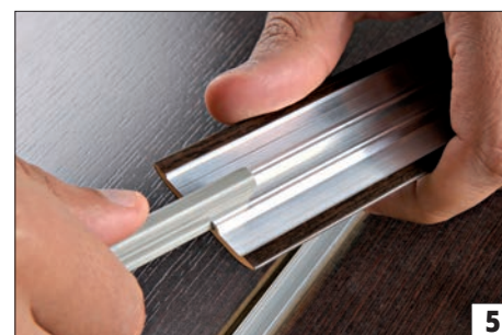
5) Keep the profile with the groove for insertion facing upwards and slot in the insert from the top downwards (if it does not slide easily, lubricate with water, silicone spray or vegetable oil).
