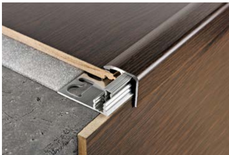
ALUM. TOP COVERED + PIN INSERT + ALUM. BASE 40 PUNCHED/PERFORATED (80 wooden finishes of which 60 on demand) thermo packed bar length 2,7 lm - pack. 20 Pcs - 54 lm (H 14 - H 16 - H 18 mm - 40,5 lm)
